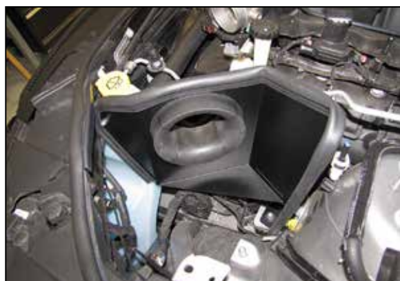
16. Install the heat shield assembly into the vehicle so the mounting grommet slides onto the inner most mounting stud. Align the heat shield with the mounting bracket and then secure with the spacer and hardware provided. NOTE: Be sure to place the spacer between the bracket and heat shield.
