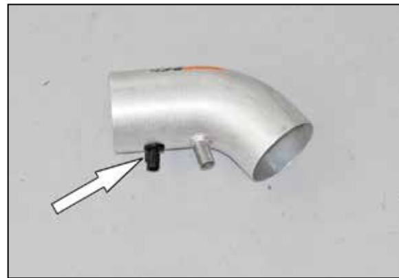
20. Install the provided grommet into the K&N® intake tube. Remove the O-ring from the inlet air temperature sensor and then install the sensor into the grommet as shown.
