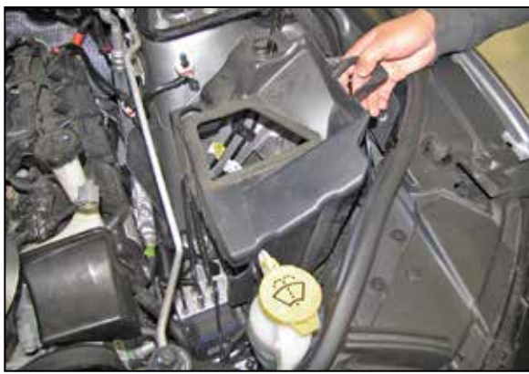
7. Lift out and remove the inlet air diverter tray from the vehicle.
