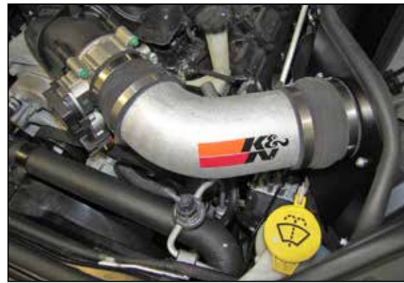
21. Install the K&N® intake tube into the hump coupler and then into the straight coupler, adjust the intake tube for best fit and then secure with the provided hose clamps.
