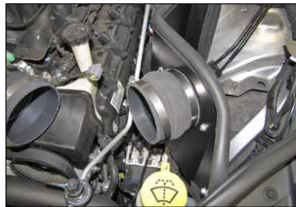
18. Install the provided coupler (08418) onto the filter adapter and secure with the provided hose clamp.
