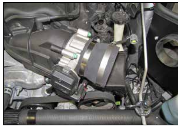
17. Install the step coupler (08497) onto the throttle body and secure with the provided hose clamp.
